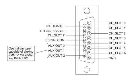
Figure 1.4 T855 D-Range 2 Wiring - Rear View (standard T800-03-0000 kit)
