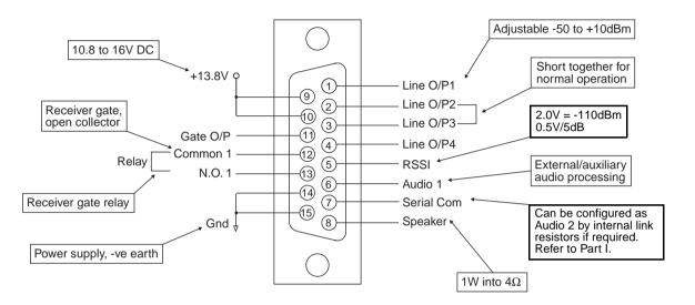
Figure 1.3 T855 D-Range 1 Wiring - Rear View
